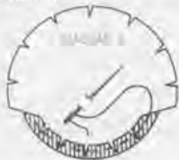
Diagram B: Clipping into the seam allowance to maintain the curved shape of the fabric piece.
